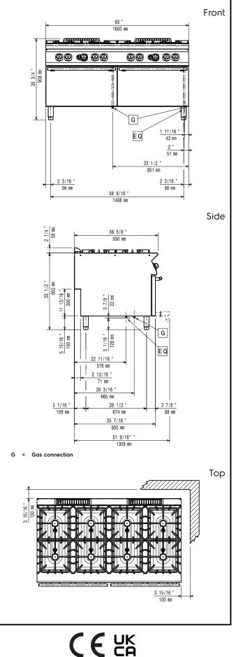
Modular Cooking Range Line 900XP 8-Burner Gas Range on 2 Gas Ovens
